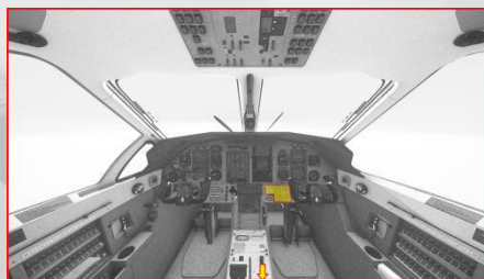
Cabin Pressurisation Control System (CPCS)
